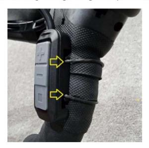
7. Loosen the handlebar tape until it reaches the shifter position. Place the wires along the shape of the handlebar, and then wrap the handlebar tape back into place.
