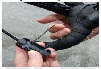
5. Place the button on the inner side of the handlebar, use pliers to hold the silicone ring, and secure it to the side groove of the button.
