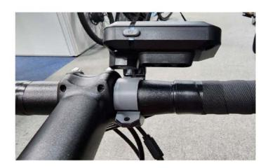
2. Use an Allen wrench to lock the console in the appropriate position on the bicycle handlebar.
