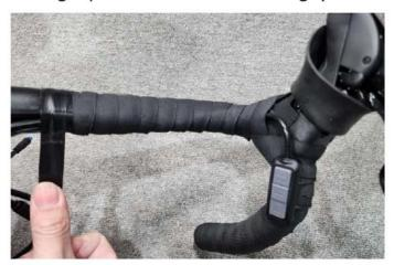
9. Reinstall the shifter rubber sleeve back to its original position.
