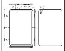
1. front camera 2. USB Type-C (charging &data transfer) 3. micro SD
