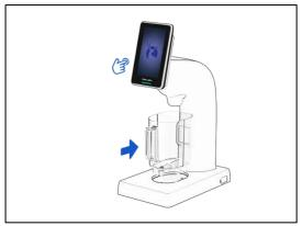
The dairy dispenser will automatically prepare according to the content of the order, and after the preparation is completed, there will be a corresponding content prompt on the screen
