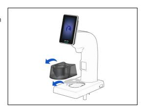
6./ The cleaning liquid tank is filled with the specified volume of cleaning liquid, and the box with the cleaning liquid is assembled on the table, and the cleaning box valve seat is connected to the joint in the sink
