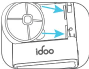
⚠️ Avoid touching the surface of the print head with your finger. Acids and oils on your skin will damage the print head.
